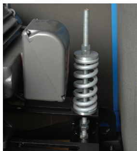
Automatic V-belt drive tensioning system.
