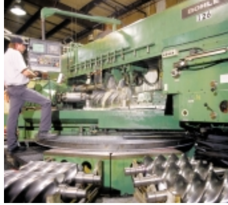
CycloBlower XP rotors are precision ground using state of the art milling technology.
