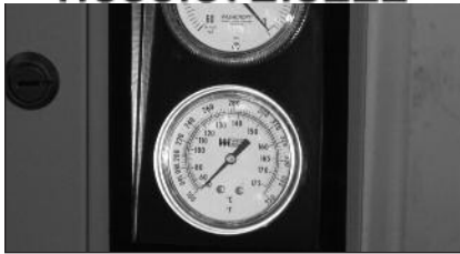
Discharge pressure, filter restriction, and temperature gauges are standard.
